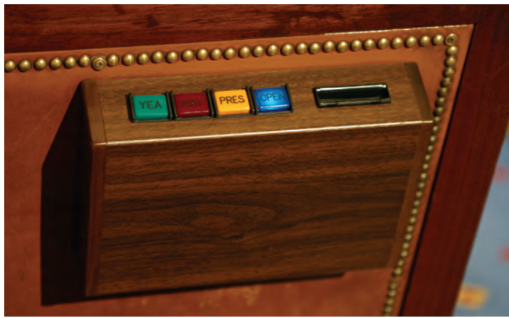
Figure 2. Input terminal for the electronic voting system. Photo courtesy of the Office of the Clerk of the House.
